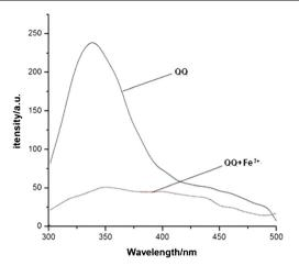
Fig 1 Fluorescence emission spectra of QQ in the presence of Fe<sup>3+</sup> in HEPES buffer solution (10 mM, pH=7.0, DMF-H<sub>2</sub>O, 9:1, v/v),  $\lambda_{ex}$ =344 nm
