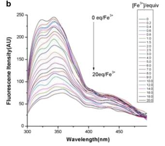
**Fig 2** a Relative fluorescence intensity changes of QQ in the presence of various metal ions(10 eq.) in HEPES buffer solution (10 mM, pH=7.0, DMF-H<sub>2</sub>O, 9:1, v/v),  $\lambda_{ex}$ =344 nm. **b** Fluorescence spectra of QQ in the
