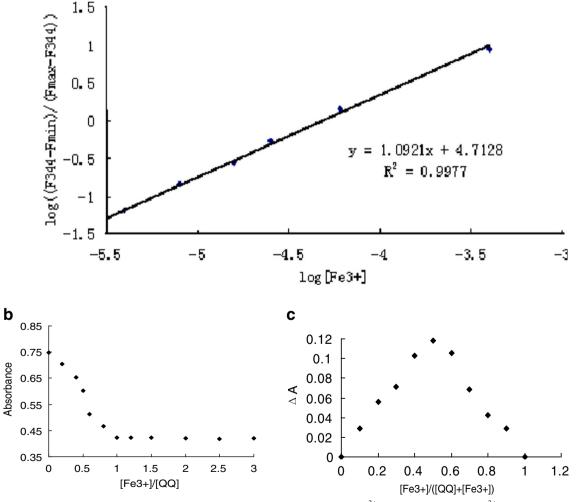
**Fig 4** a Curve of fluorescence intensity at 344 nm of QQ versus increasing concentration of Fe<sup>3+</sup>. b Absorbance of QQ-Fe<sup>3+</sup> complex in different [Fe3+ /[QQ] ratio. c Job's plot for the QQ-Fe<sup>3+</sup> complex ( $[QQ]+[Fe^{3+}]=5\times10^{-5}$  mol dm<sup>-3</sup>)
