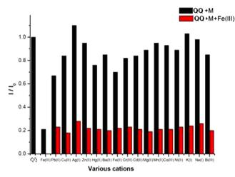
Fig 3 Relative fluorescence intensity changes of QQ in the presence of various metal ions (20 eq.) and Fe<sup>3+</sup> (20 eq.) in HEPES buffer solution (10 mM, pH=7.0, DMF-H<sub>2</sub>O, 9:1, v/v). $\lambda_{ex}$ =344 nm
